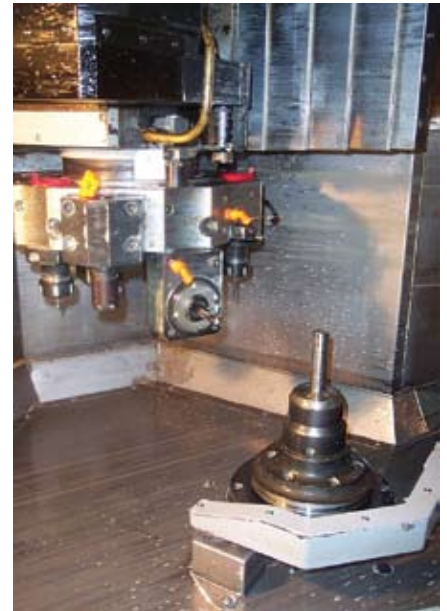
A view of a live tool inside the Haas SL-20 multitasking lathe.
