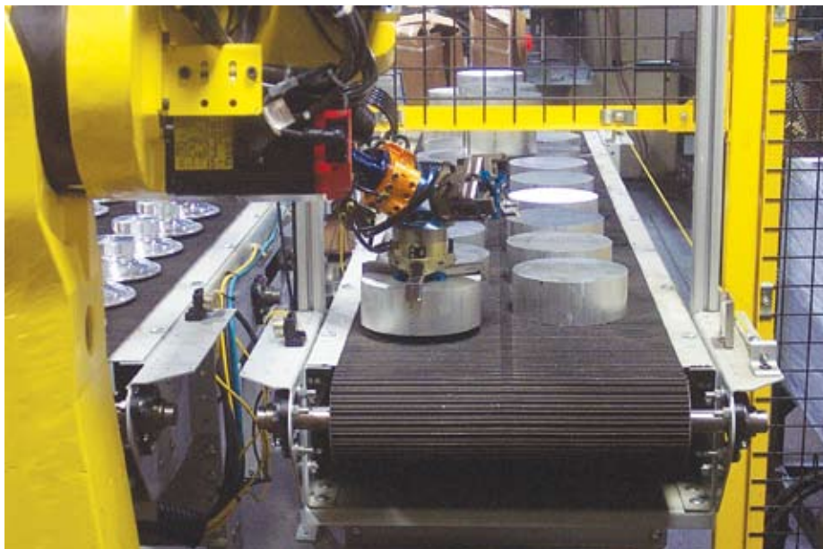
A robot picks up a slug from a conveyor to be placed in a Nakamura WT-300 multitasking lathe at TMCO.
