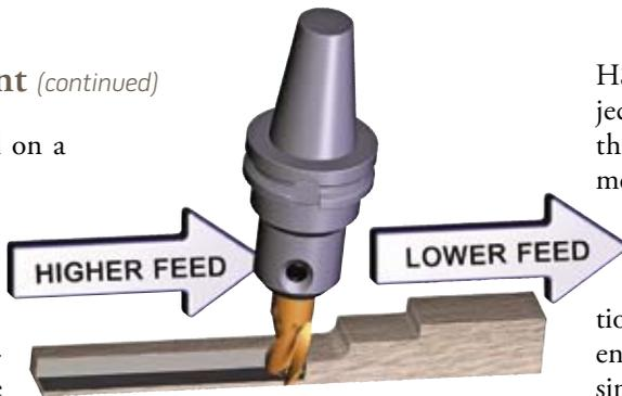
**Figure 5:** In high-speed CAM strategies, if the tool is approaching a step, software will slow the tool feed rate down. After the step, the CAM software will increase the feed rate to the maximum allowable.
