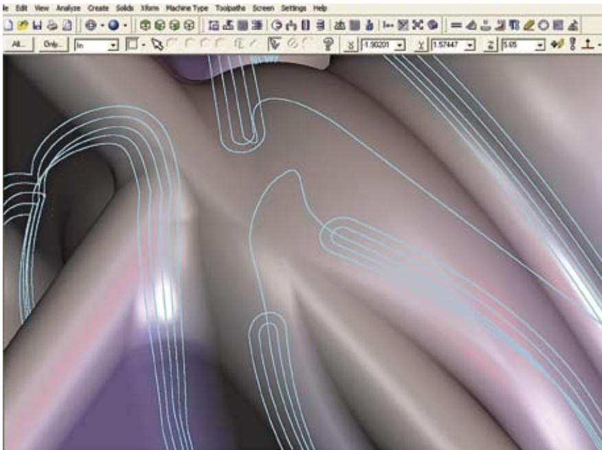
Figure 4: Constant Z toolpaths tend to leave chunks of material between adjacent surfaces. The pencil toolpath will clean these areas, leaving a smooth radius between the surfaces.
