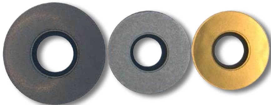
Green (left), sintered (middle) and coated (right) inserts show the dimensional change from green to sintered WC.
