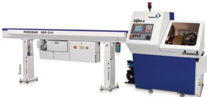
Tornos reports that its DECO Sigma 8 CNC automatic lathe provides a diameter accuracy of \pm 1\mu\text{m} .
