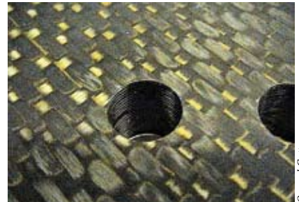
Example of a clean hole entry when drilling a carbon-fiber composite material.
