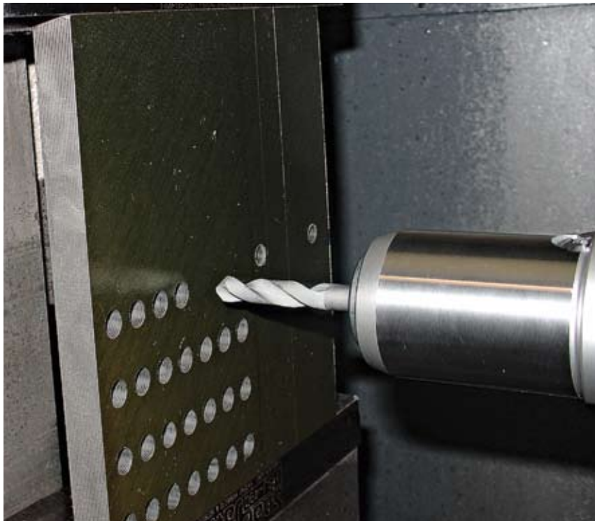
In a test conducted by Kennametal, the toolmaker's Split-Point Fiber drill produced 300 through-holes in difficult-to-machine carbon fiber-reinforced polymer composite before burrs formed and delamination occurred compared to 150 holes for a PCD-veined drill.
