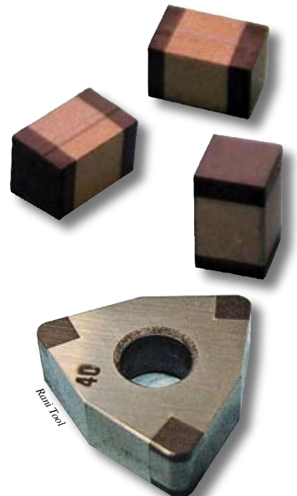
Pressed PCBN/carbide/PCBN “sandwiches” (top photo) can be brazed into insert corners (above) in a single operation, reducing tool manufacturing costs. The resulting inserts, like these from Rani Tool, are less expensive, and inserts with negative geometries can be flipped to permit machining with both sides of the tool.
