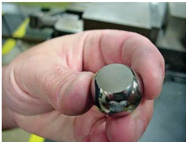
A modified ball bearing is used to apply pressure to the center of the vise and the center of rough sawed stock.
