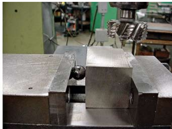
A modified ball bearing is used to apply pressure to the center of the vise and the center of rough sawed stock.
