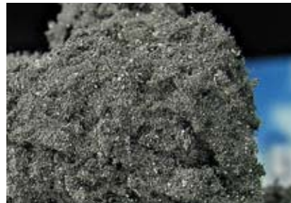
This magnified image of the swarf produced by CF grinding reinforces the concept of micromilling. Note how the individual particles interlock like steel wool, the result of creating long, stringy chips.
