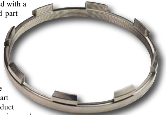
CF grinding generated the slots and chamfers from a solid without producing burrs.
