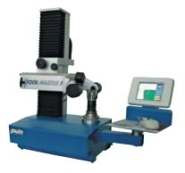
**REGO-FIX TOOL CORP.**, Indianapolis, introduced a new TCAM2 monitor for its Toolmaster 10 presetter. The Toolmaster 10, made by Rego-Fix and PWB Systems AG, Switzerland, is a manually operated bench model. Its measuring column and tool spindles are mounted on a thermally stabilized and stress-free cast iron base. TCAM2 uses a digital CMOS camera. Maximum Zaxis measurement for two Toolmaster 10 models is 360mm and 500mm.
