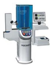
**HAIMER USA LLC**, Villa Park, Ill., introduced its Tool Dynamic presetter combined measuring and balancing system. It uses saturn 1 image processing technology and a telecentrical objective camera with 35× magnification and automatically recognizes the shapes of cutting edges. Maximum Z-axis measurement is 450mm.
