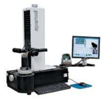
**BIG KAISER PRECISION TOOLING INC.**, Elk Grove Village, Ill., recently introduced the Speroni STP-35 Basic and STP-35 EzVision tool presetting systems. BIG Kaiser is the exclusive North American distributor of Speroni presetters. The new benchtop system has an extended Z-axis height to accommodate tools up to 20" (500mm) in length and display resolution of 0.000039". The optional EzVision is an automatic, digital tool sensing and measurement system.
