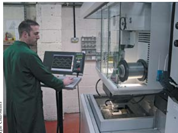
An operator prepares a program on a high-accuracy Vertex EDM for cutting a die insert that will be used in a progressive die for semiconductor production.
