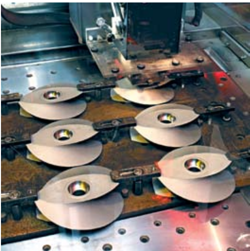
Intricate EDM faces poor flushing conditions with these Stellite workpieces. The machine shop compensates for the conditions and can therefore increase cutting speed by applying Makino's HEAT, an EDM technology specifically developed for EDMing workpieces in poor flushing conditions.
