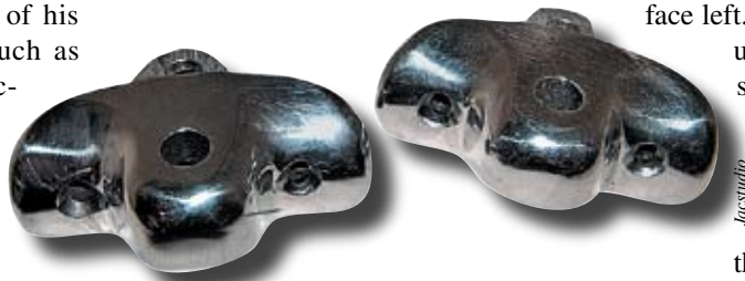
Jac Corless machined these highly contoured aluminum housings and fabricated the windshield-wiper transmission components they contained for a 1936 Buick undergoing restoration.
