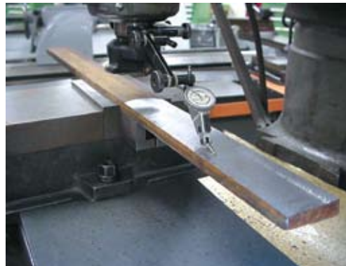
To remove the warp on a long bar clamped with a vise, each cut section must be indicated flat before proceeding with the next cut.
