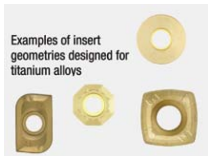
Examples of insert geometries designed for titanium alloys In machining titanium, cutter bodies and inserts must use very positive cutting angles to achieve progressive cutting action and avoid impact.
