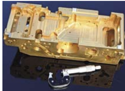
Machining this approximately 4"×5"×14" aluminum component at The Manufacturing Facilitators required more than 600 operations, some of which tested the accuracy limits of the machine tool itself.
