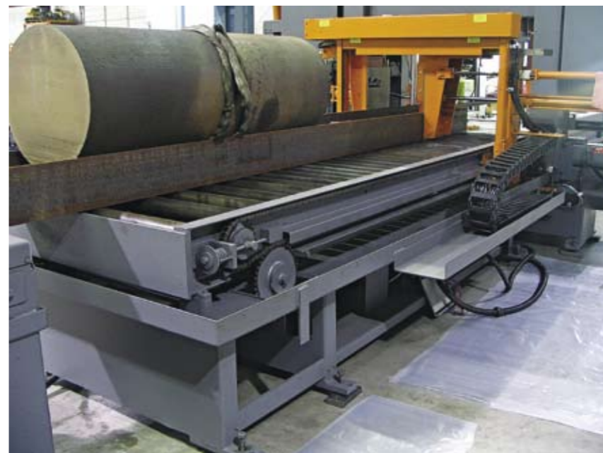
HE&M's "Steel Service Center" system is a long-stroke, hydraulic shuttle-positioning system that automatically indexes to a preprogrammed length for a preprogrammed quantity of parts. Positioning material via the shuttle-feed system frees the operator from repositioning materials after each cut.
