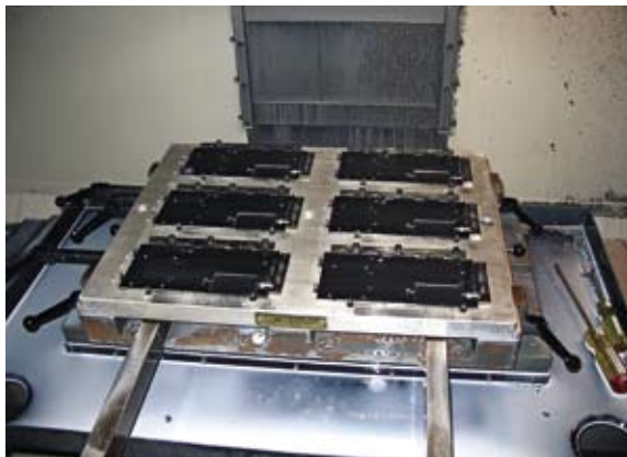
A Steel Craft pallet loaded with six substrates installed in Haas VF-0 at Ceramics Process Systems. Spring-loaded pins hold the parts as they undergo only light machining.
