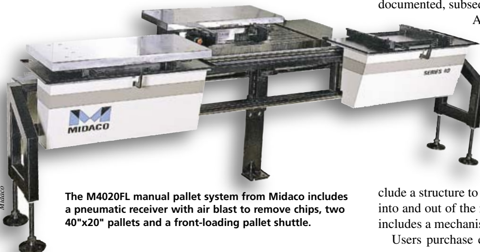
A Midaco automated pallet system uses pneumatic clamping and clears chips from the contact pads with a blast of air when moving a pallet into place. This pallet system has its own controller, which automatically responds to the machining center's request for a pallet change. Midaco produces systems with pallet sizes from 10"x12" to 29"x120".
