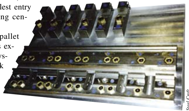
A typical fixture setup on a Steel Craft pallet. This setup shows two sets of fixtures for two different parts. For economy, a single pallet can be set up for multiple parts.
