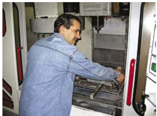
Ceramics Process Systems Manufacturing Manager Mike Boucher installs a manual pallet loaded with parts into a Haas VF-0.
