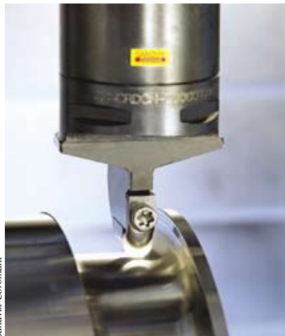
An aerospace component made of 718 Inconel is machined with a new ceramic SiAlON insert grade from Sandvik Coromant.
