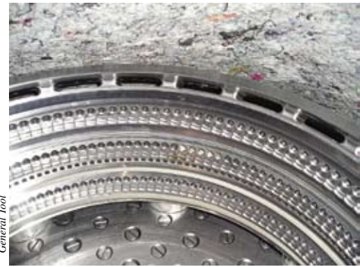
This prototype engine stator case, made of Greek Ascoloy stainless steel, was machined at General Tool Co. on a 5-axis Deckel Maho machining center fitted with a right-angle head.
