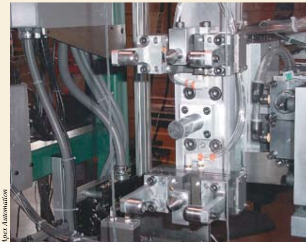
A semiautomatic pick-and-place loader for a pipe-fitting tapping machine automatically transfers fittings from a conveyor to the fixture in a machining center. However, an operator loads the fittings onto the conveyor.
