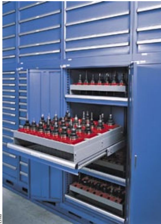
Stacked modular cabinets store tools in protective molded holders.
