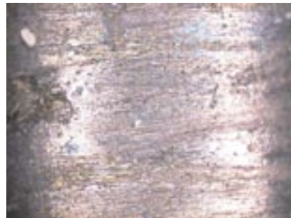
Finish inside of a titanium-composite stack hole drilled with a diamond-coated carbide drill.
