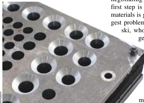
Stacked material drilled with countersunk holes.
