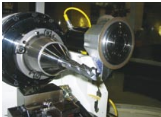
Walter Helitronic Power grinding machine with a BPR diamond profiling roll mounted onto a DC brushless dressing spindle. The workpiece is a 3/4" 4-flute carbide endmill.
