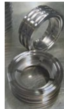
By supplementing a standard group of tools that stay on the machine with additional tools to produce specific part features, CNC Industries efficiently machines 12L4 mild-steel hydraulic components (inset) on a Mazak Super Quick Turn 15 CNC lathe (above).
