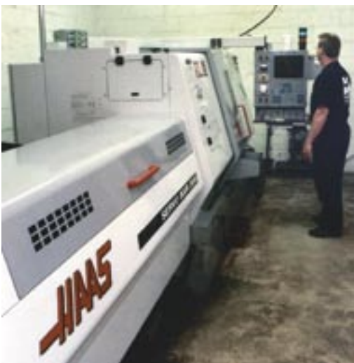
Jeff McGaffic checks the control of the Haas TL-15 dual-spindle lathe at his Vista Manufacturing shop. The machine features a bar feeder that permits unattended operation and helps maximize machine uptime.
