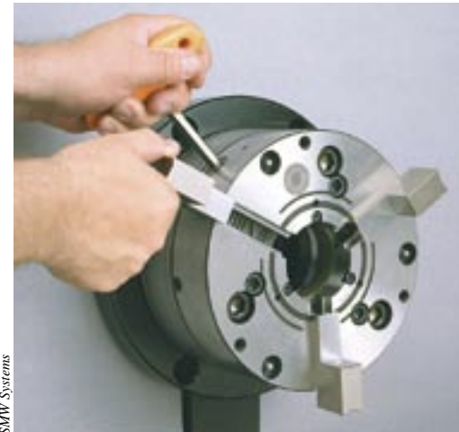
A quarter-turn of the hex key lets these jaws from SMW Systems adjust to any position.
