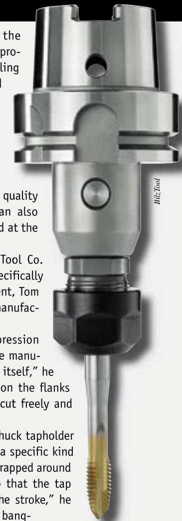
Synchro Chuck tapholders feature an oil-repellent polymer wrapped around the cross post, which prevents the tap from tearing the thread at the bottom of the stroke.
