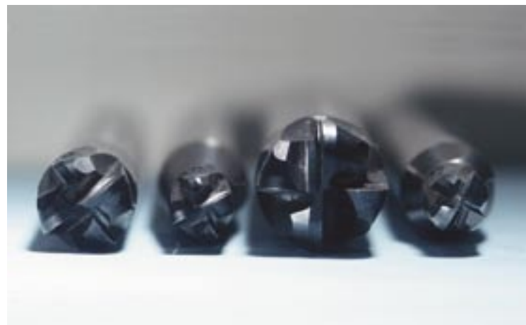
A selection of 4-flute ball and flat-bottom solid-carbide cutting tools from Current River Die Sinking’s Tribute series.
