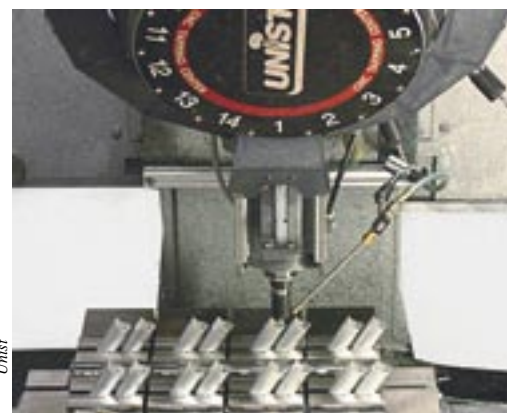
Sixteen saw nozzles are milled while an external dry-machining nozzle applies lubricant.
