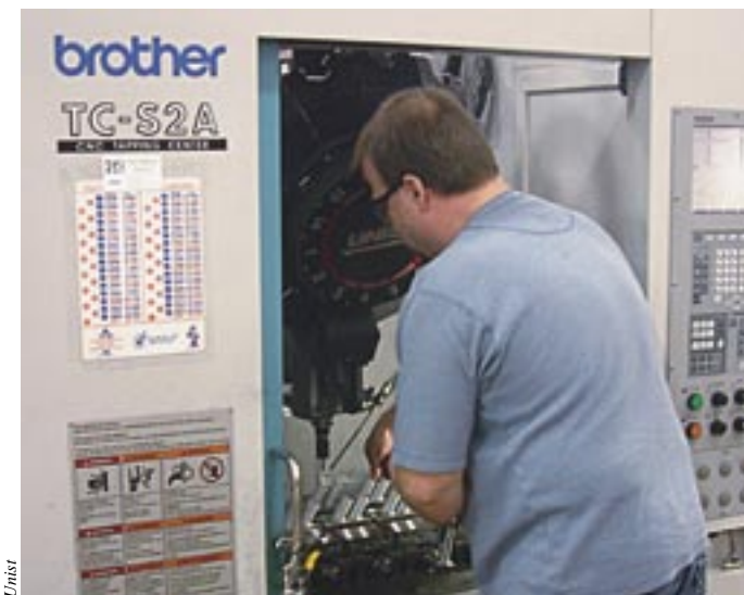
A Unist machinist loads parts into a Brother CNC machine to perform near-dry machining.
