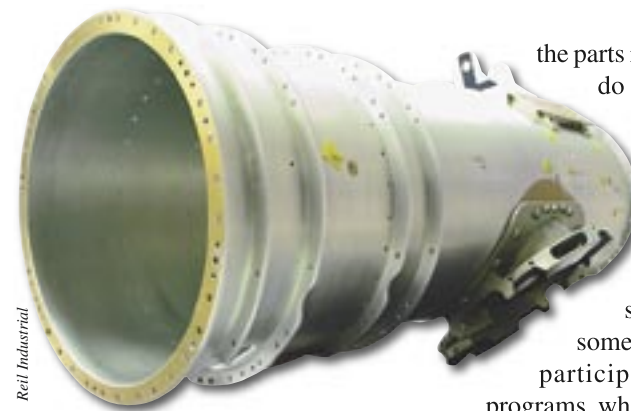
Forward transition component of the space shuttle's robotic manipulator system—the Canadarm.
