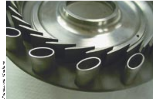
This complex 10.67"-dia. nozzle plate, machined from solid titanium, is an air-conditioning component for the new Airbus A380 jumbo jet.
