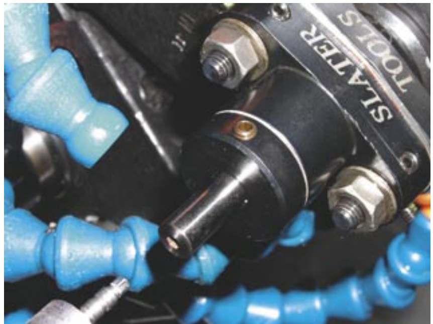
An example of external rotary broaching.
