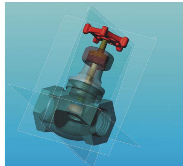
Three-D CAD software allows various sections of this globe valve to be viewed, as well as its overall design.
