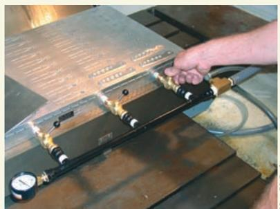
**An operator releases completed workpieces by simply turning the handle on a vacuum chuck valve by 90° to the “off” position.**
