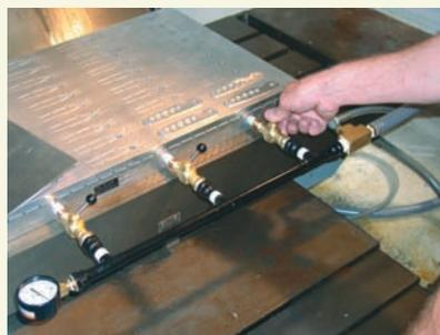
**An operator releases completed workpieces by simply turning the handle on a vacuum chuck valve by 90° to the “off” position.**
