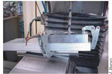
One way to easily machine a feature on a compound angle is to use a simple universal angle fixture.
