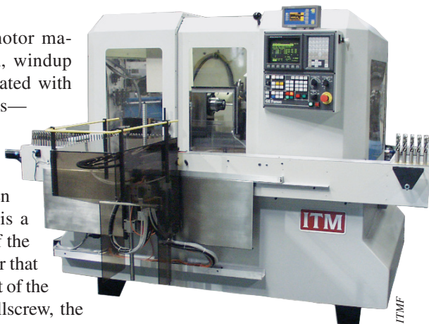
International Tool Machines of Florida's Series 2005-THG thread grinder.
