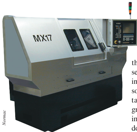
The MX17 universal thread grinder's wheel and dresser operate in the same plane, which helps ensure accuracy of the final thread form and reduce dressing time.
