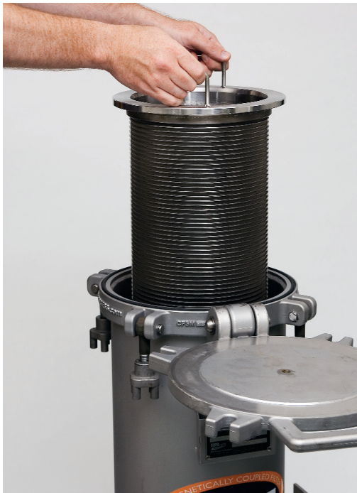
Removal of the filter core from a magnetically coupled filter is the same as with most cartridge filters, but it needs to be removed less frequently because it incorporates self-cleaning technology.
