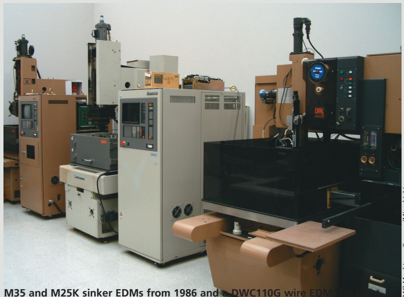
M35 and M25K sinker EDMs from 1986 and a DWC110G wire EDM from 1984 housed in the museum.
