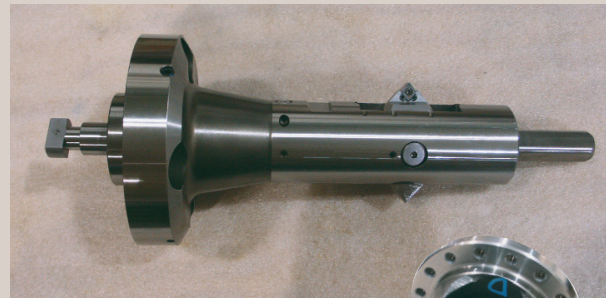
The Mapal drawbar-actuated tool, with PCD insert, feeds out into the ductile iron casting and finishes the four internal spherical surfaces of the differential case (inset).
