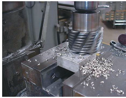
For rough milling, it’s hard to beat a short, beefy corncob-type cutter.
