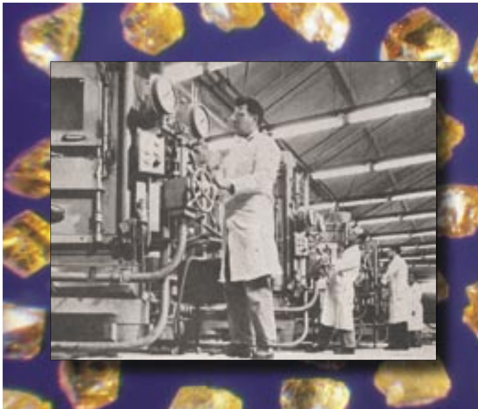
Engineers regulate the machine used to produce Man-Made industrial diamonds at General Electric's Metallurgical Products Dept.
