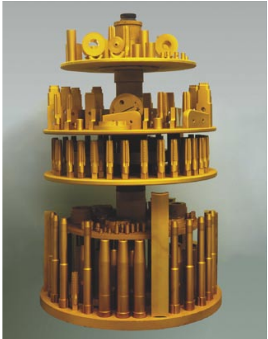
Pipe taps and assorted components being CVD-coated.
