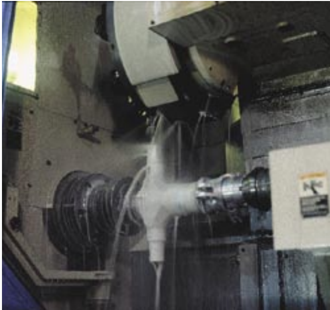
Multitask machines minimize moving parts from machine to machine.
