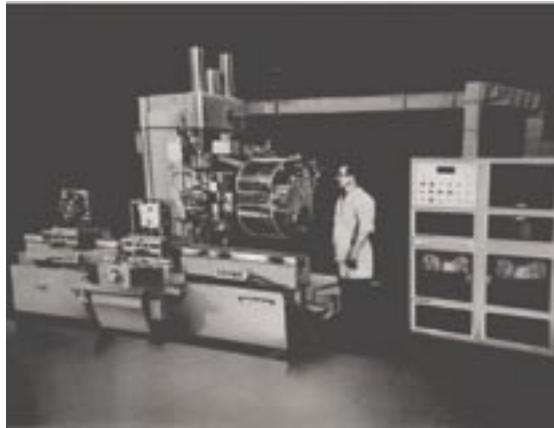
Kearney & Trecker's 1958 Milwaukee-Matic II NC machining center featured an automatic toolchanger.
