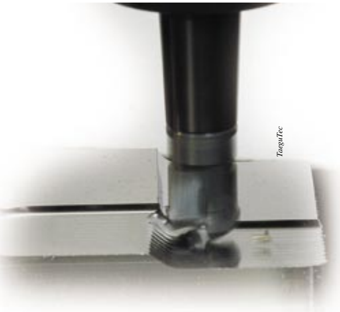
A button cutter is used for HSM.
