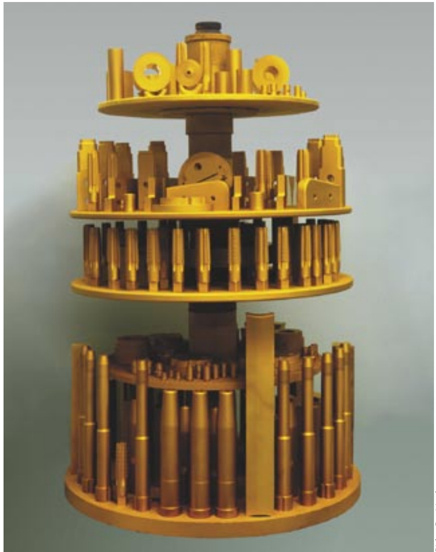
Pipe taps and assorted components being CVD-coated.
