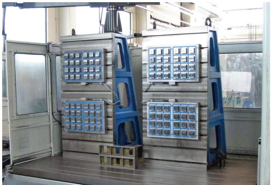
A set of four 20"x32" NG100 magnetic chucks on angle plates for large mold components with a part mounted (left) and without.
