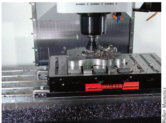
Permanent-magnetic chucks provide uniform part-gripping pressure when milling, which reduces machine-induced vibration.
