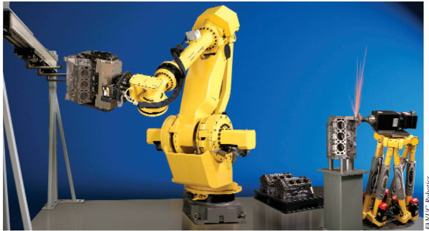
Example of an industrial robot with a large payload capacity (left) and one for performing metal removal.
