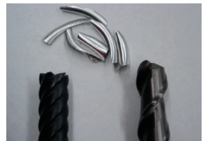
Long and large aluminum chips are created from a ductile material. The shallow flutes of the tool on the left would clog and cause the tool to fail.
