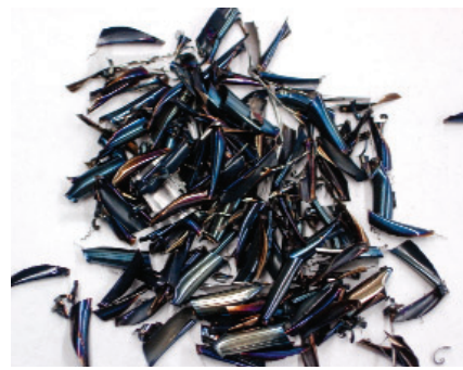
Regarding thermal conductivity, chips from 4140 steel show heat transported to the chips. The color change indicates a high level of heat contained in the chips.
