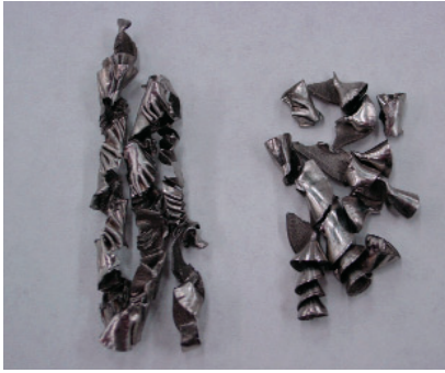
Identical drilling applications involving 316 stainless steel result in different chip formation due to geometrical differences in tools.
