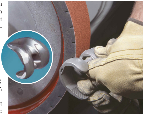
Manual finishing of a knee implant. Inset: The use of cobalt chrome for artificial knees and other implants is growing because of the material's resistance to wear.
