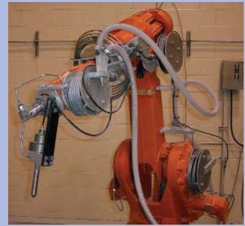
Robot fitted with an AWJ cutting head at Chukar Waterjet.
