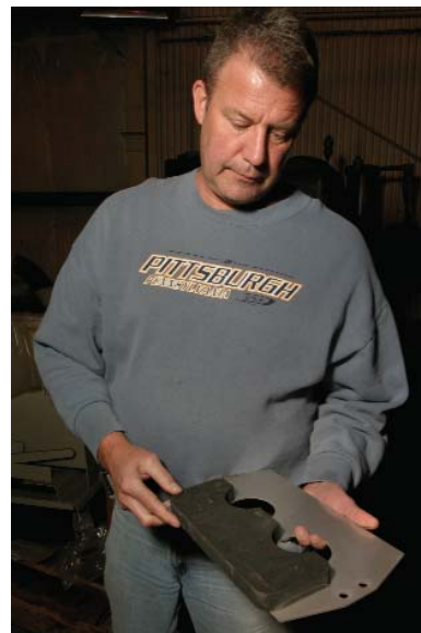
Tom Green, owner of Kutz Fabricating, shows mating rubber and stainless steel conveyor components that were cut, separately, on an AWJ machine.
