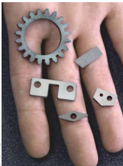
Blanks for these small HSS parts were cut on an AWJ machine at Arthur R. Warner Co.
