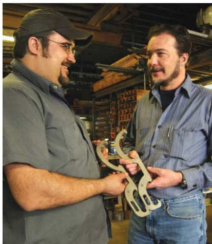
Mike Warner, president of Arthur R. Warner Co. (right), and Mathias Packe, shop supervisor, inspect stainless steel hose wrenches cut on an AWJ machine.
