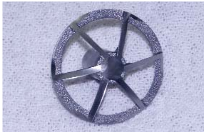
Stainless steel shoulder cutter.
