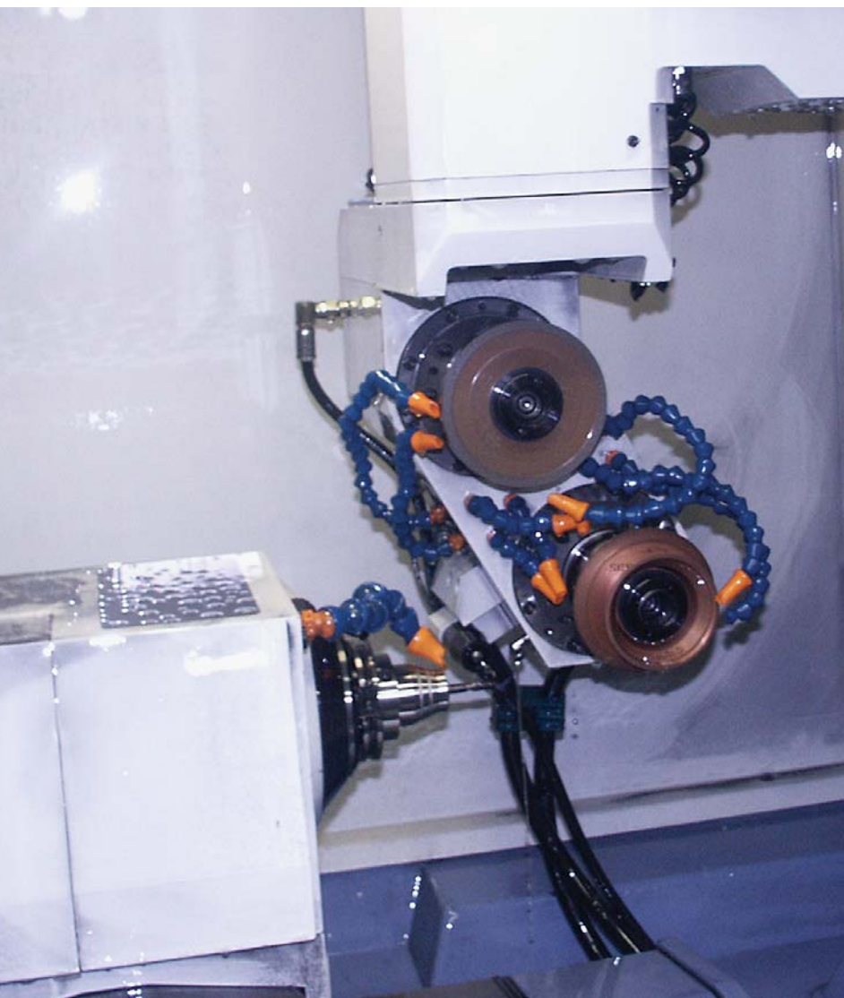
Oak View Tooling grinds a tool on an Anca RGX grinder.
