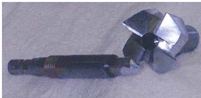
Stainless steel orthopedic cutting tools.
