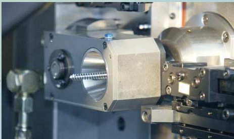
Thread-whirling capabilities on Swiss turning machines permit creation of acute thread profiles in difficult-to-machine materials without the need for secondary operations.
