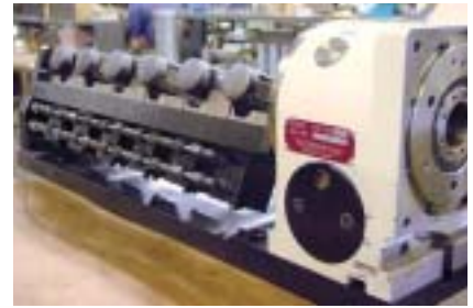
The Tsudakoma RN-150R is a 6"-dia. rotary table used to rotate the attached trunnion-style fixture with tailstock support and baseplate.
