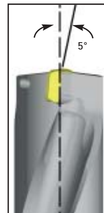
Figure 3: A positive rake angle helps direct chips up the flute, aiding in chip evacuation.
