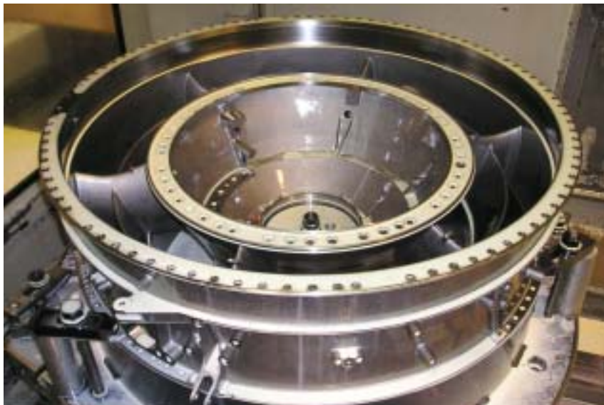
Mechanical clamps constrain this titanium jet engine fan frame for machining.
