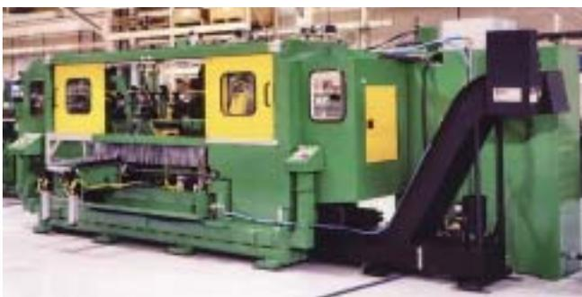
Bardons & Oliver starts with a base machine of a certain size and a selection of spindle and chuck sizes and customizes the equipment based on the application requirements.
