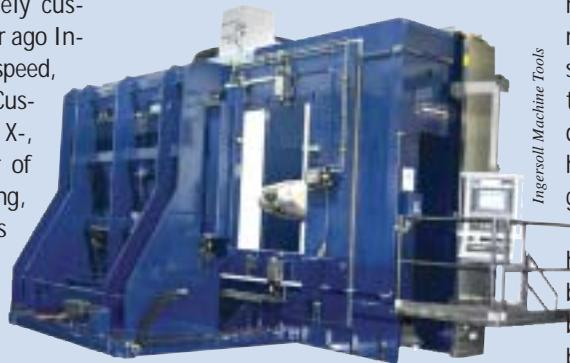
**When selecting a machine from Ingersoll’s line of profile-type milling machines, customers are able to specify the X-, Y- and Z-axis strokes, number of tool-magazine modules, fixturing, and spindle speed and power, as well as choose from an array of parts-handling systems.**
