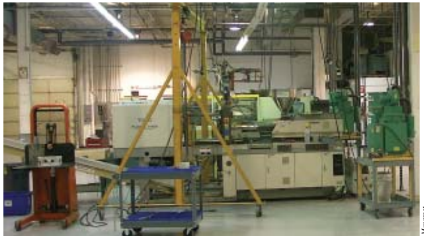
Standard thermoplastics injection machines are used for MIM.
