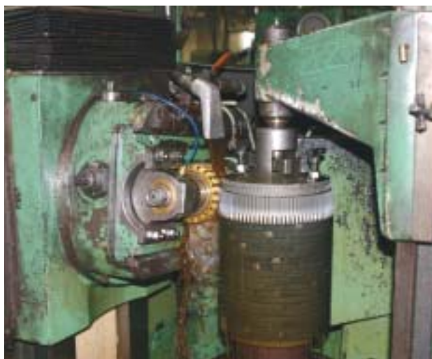
A hob cuts a starter ring using SoyEasy-UNICut.
