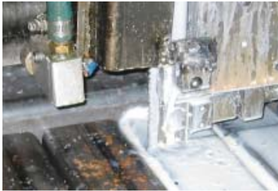
A bandsaw cuts tubular steel using SoyEasy-Cool.
