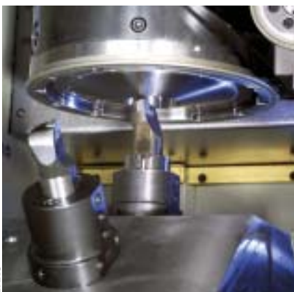
Turn/grind processing of a hardened variable-speed pulley, hardened to 58 to 62 HRC, on an EMAG Reinecker VSC 250DS includes hard preturning the pulley surface with a CBN-tipped insert (left), peel grinding the surface with a CBN wheel (center), and finish grinding two internal bore diameters with sintered corundum (right).
