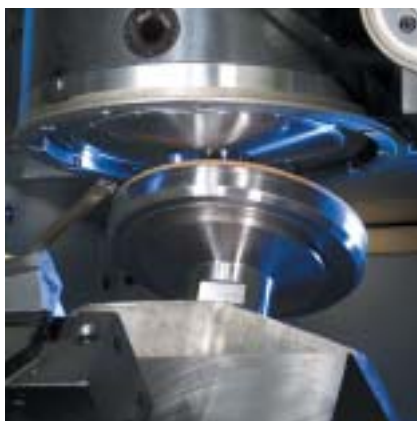
Turn/grind processing of a hardened variable-speed pulley, hardened to 58 to 62 HRC, on an EMAG Reinecker VSC 250DS includes hard preturning the pulley surface with a CBN-tipped insert (left), peel grinding the surface with a CBN wheel (center), and finish grinding two internal bore diameters with sintered corundum (right).
